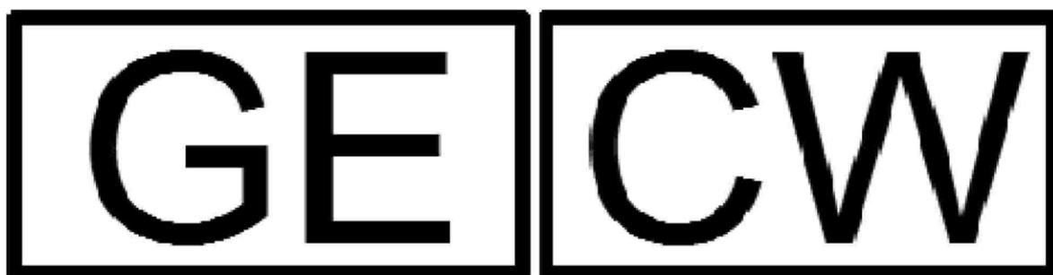
The letters shall be of the same font type as the TEN marking. The size of the letters shall be at least 100 mm high. The outer measures of the frame shall be at least 275 mm wide and 140 mm high, the frame shall be 7 mm thick.
