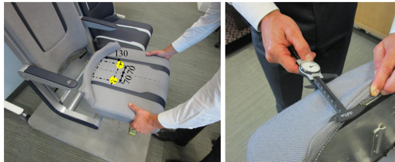
Figure 26: Seat Pad Thickness Measurement
