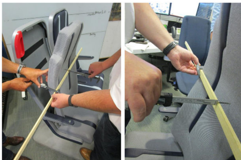
Figure 27: Back pad thickness measurement
