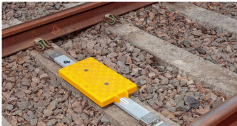
Example of a typical balise
