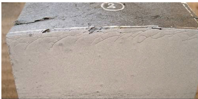
Figure 35: Section through a wheel with RCF
