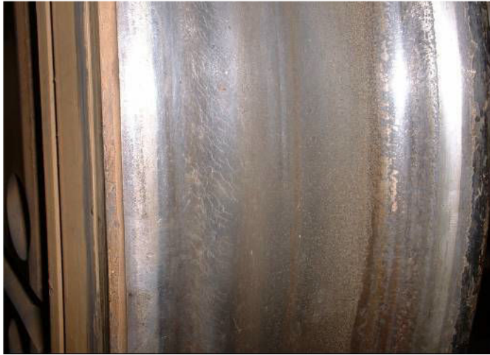
Figure 34: Light cracking due to RCF
