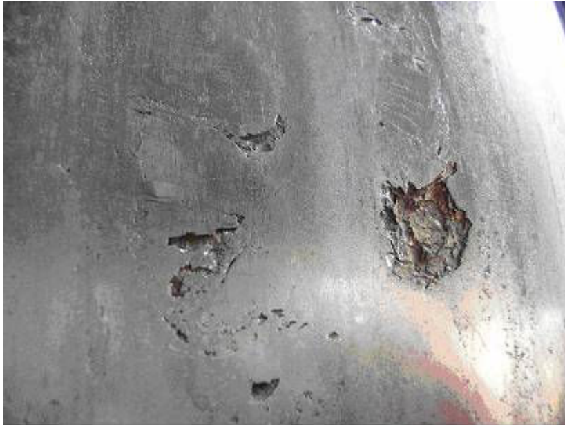
Figure 36: Typical damage associated with a wheel slide showing cracks and spalling
